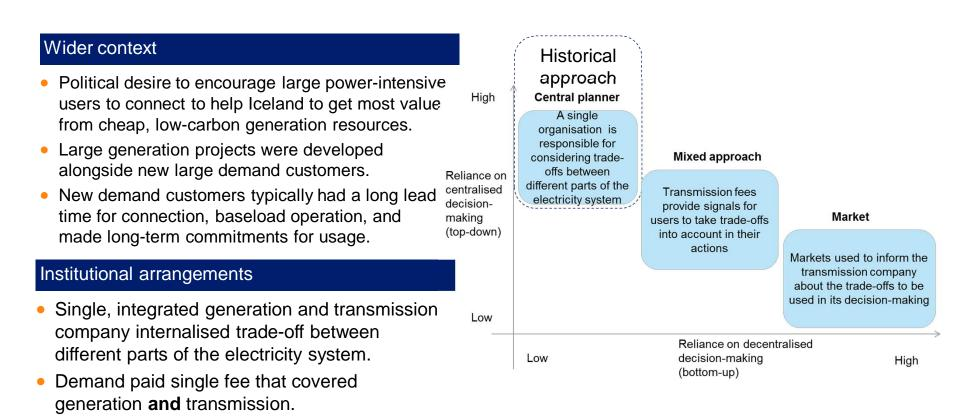
**Result:** System with 'adequate' capacity based around large, long-term, predictable customers (generation and demand)
